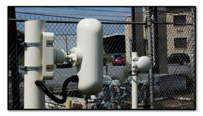
The **Predix**<sup>™</sup> detector is a linear barrier based on K-band microwave technology. It is comprised of a transmitter and receiver, which together establish perimeter protection with coverage up to 300 meters. It is very simple to install, yet provides a high level of security performance. The microwave signal is digitally converted and analyzed by a microprocessor using an innovative and efficient algorithm.
